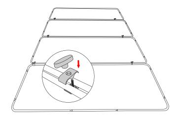
3 Use hinge clips to connect two frames.
