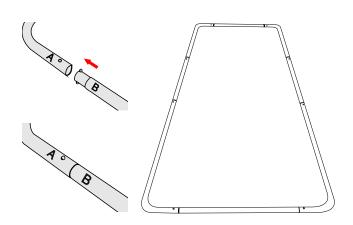
Please connnect tube A with tube B by pressing down the spring pin,until it is bounced back.
