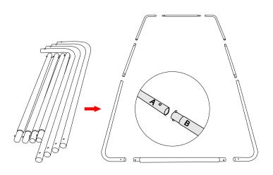
Each frame is combined by 4pcs straight tubes-A and 4pcs curved stubes-B. (As picture).
